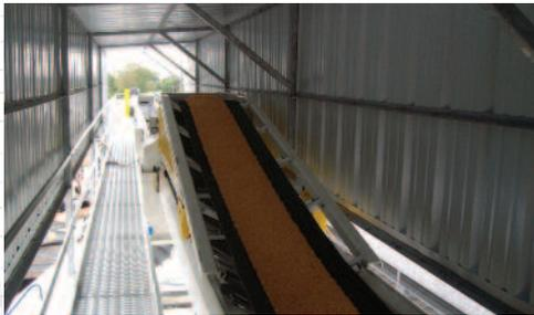
materials allow, a tripper may be designed without supporting the belt as it inclines up and out of
