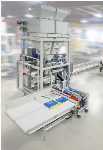
Chantland duplex bag filling scale and AP2300 bag placing system during factory acceptance test prior to shipment.
