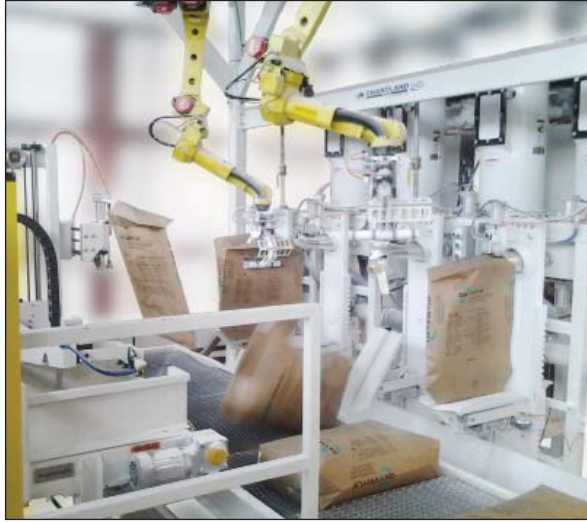
Chantland uses Fanuc Robots in some systems to place valve bags on pneumatic bag filling scales, as shown in operation at a customer facility.
