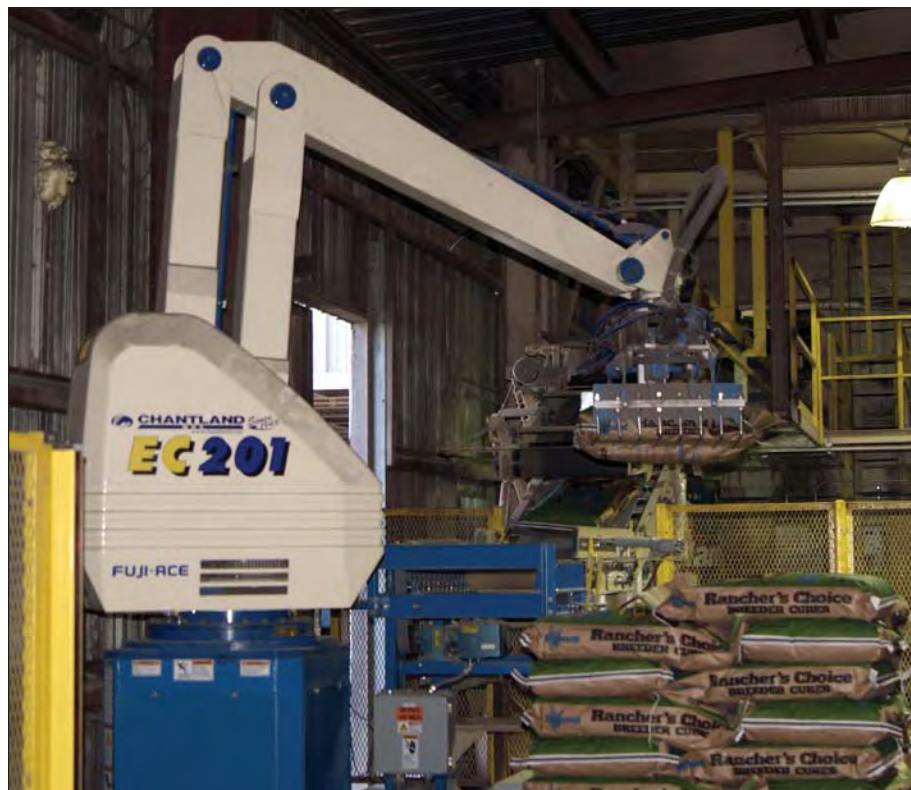
One of three new Chantland Fuji-Ace robotic bag palletizers in operation, capable of stacking in excess of 20 bags per minute.
