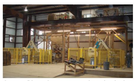
The two parallel mixing lines can operate simultaneously and package the cement and masonry mixes in either paper valve bags or open-top polypropylene bulk bags.
