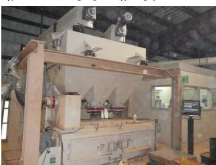
The 110-cubic-foot-capacity horizontal batch mixer with eight Shearmakers has a 7,000-pound-batch capacity and can produce nonsanded gray cement mixes at up to 25 t/h.
