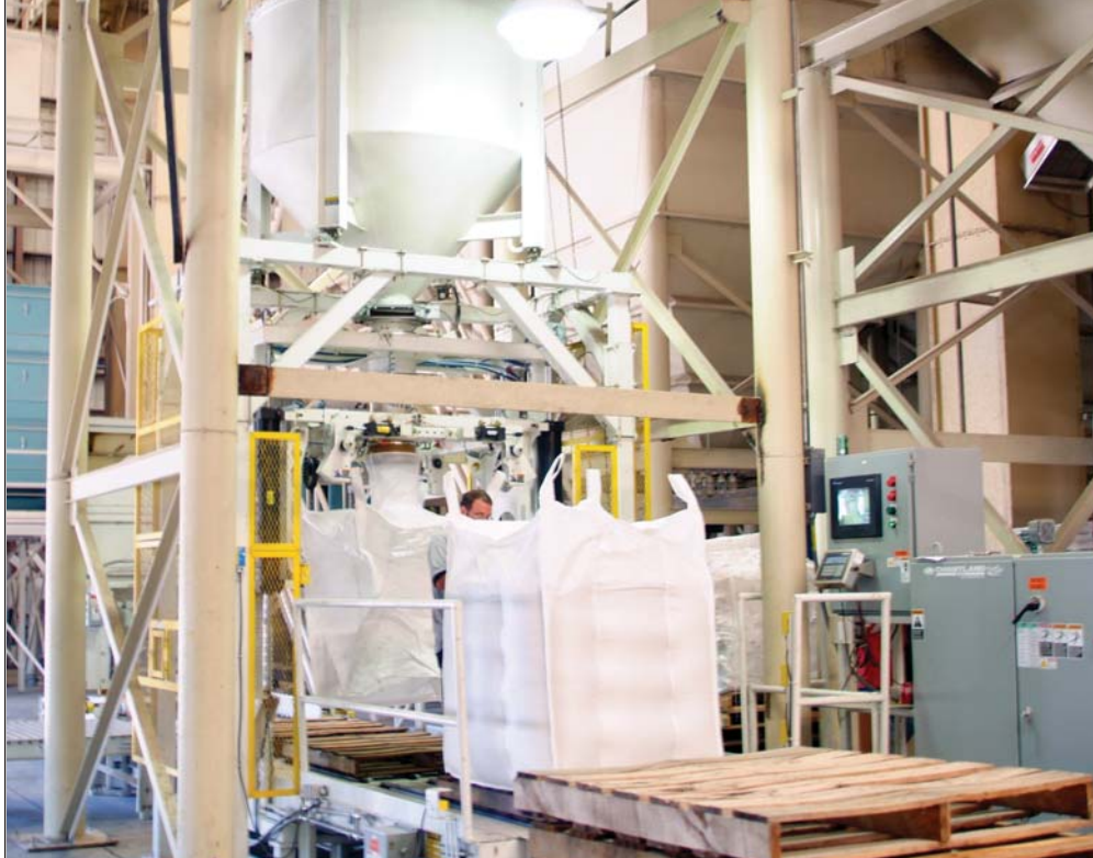
An operator inspects a filled bulk bag as the Chantland 4360 automated bulk bag filler automatically fills the next bag. By raising the baffled bag above the pallet during filling, bags are more densely filled and deform less during warehouse storage.
